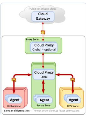
The left option, which has multiple local cloud proxies, could be preferred when one site is involved, that is, the local and global cloud proxies are deployed on the same site and communicate within the site. This enables a more logically separated deployment.
